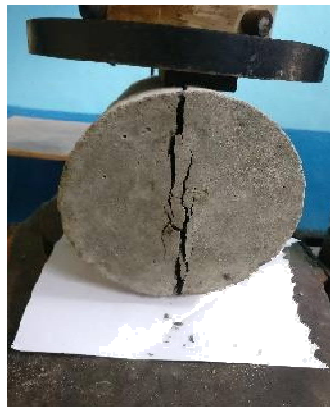
Fig 6.2 Split Tensile Strength Test
